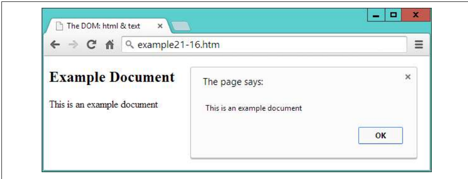
Figure 21-14. Retrieving and displaying the HTML of an element
