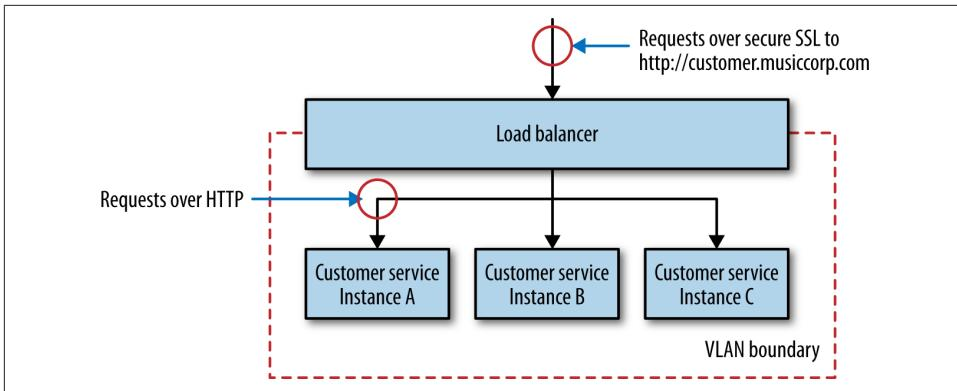
Figure 11-5. Using HTTPS termination at the load balancer with a VLAN for improved security
