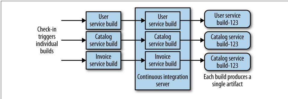
Figure 6-3. Using one source code repository and CI build per microservice
