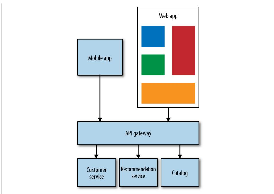
Figure 4-9. Using a single monolithic gateway to handle calls to/from UIs
