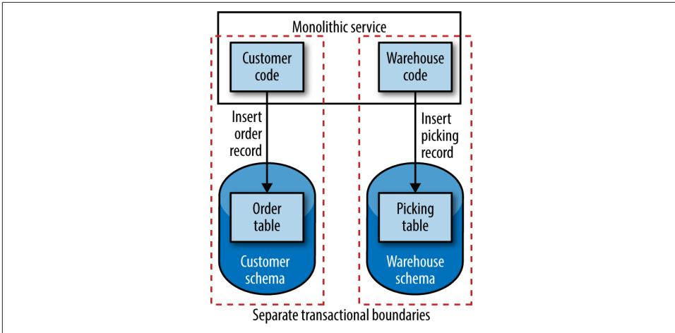
Figure 5-11. Spanning transactional boundaries for a single operation
