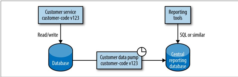
Figure 5-13. Using a data pump to periodically push data to a central reporting database
