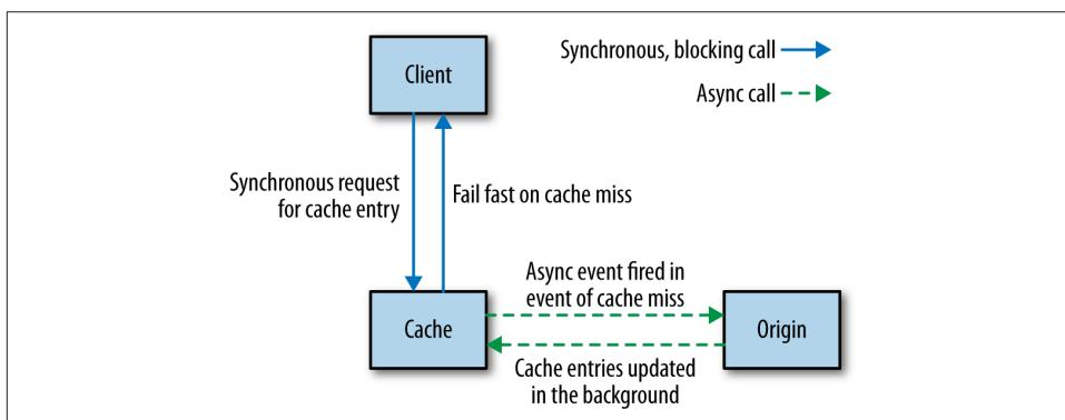
*Figure 11-7. Hiding the origin from the client and populating the cache asynchronously*
