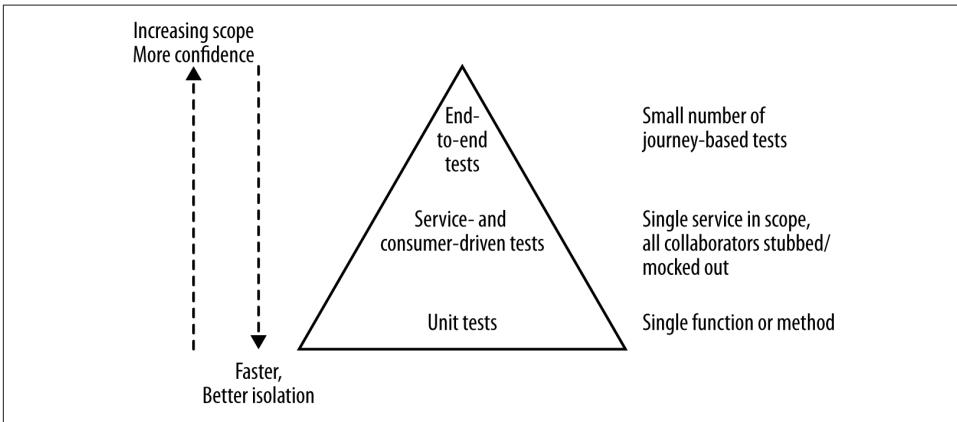
Figure 7-10. Integrating consumer-driven tests into the test pyramid
