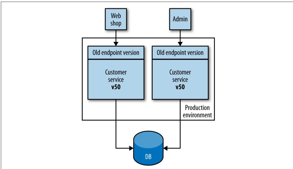
*Figure 4-6. Running multiple versions of the same service to support old endpoints*
