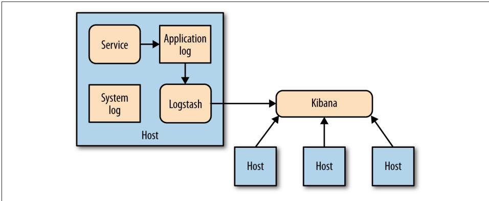
Figure 8-4. Using Kibana to view aggregated logs
