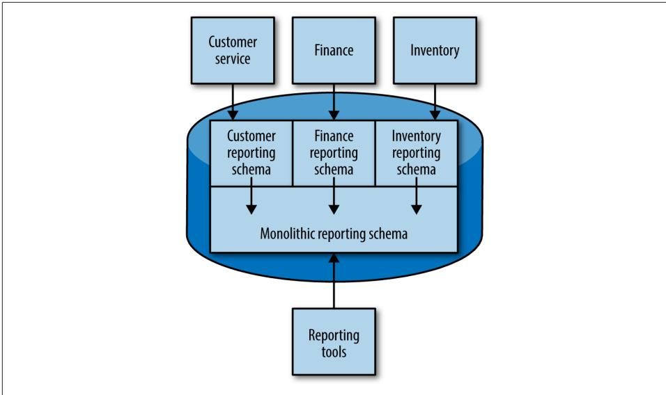
Figure 5-14. Utilizing materialized views to form a single monolithic reporting schema
