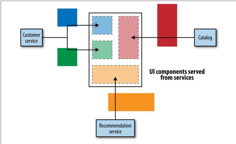
Figure 4-8. Services directly serving up UI components for assembly
