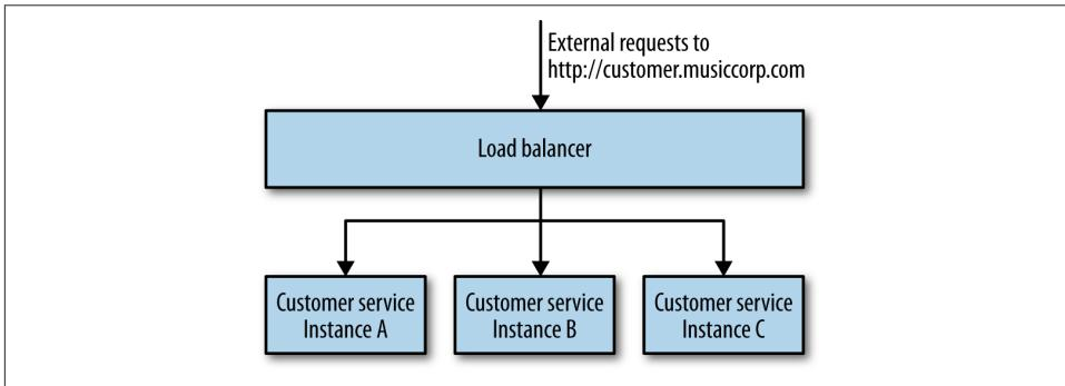
*Figure 11-4. An example of a load balancing approach to scale the number of customer service instances*
