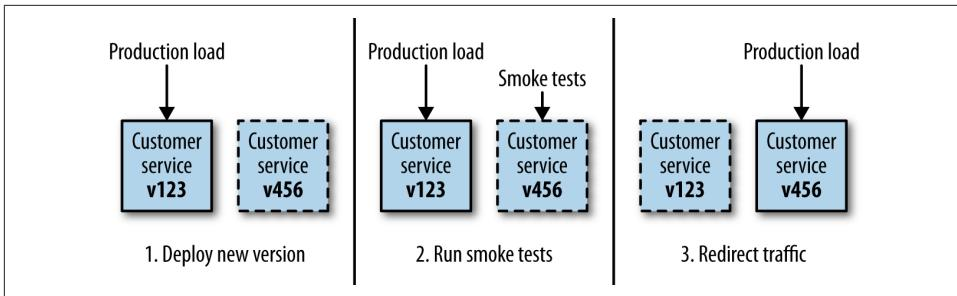
Figure 7-12. Using blue/green deployments to separate deployment from release
