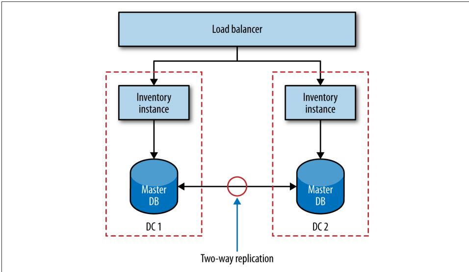
Figure 11-8. Using multiprimary replication to share data between two database nodes
