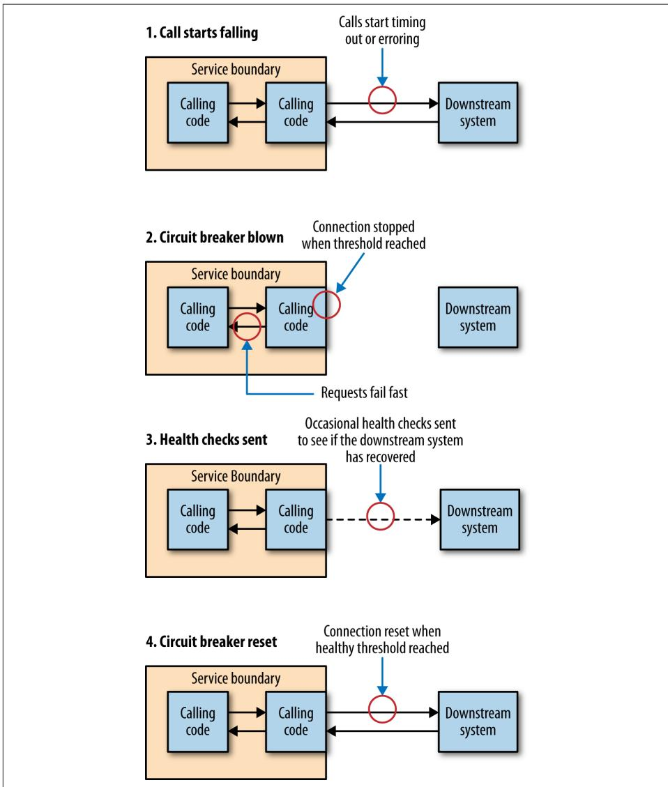
Figure 11-2. An overview of circuit breakers
