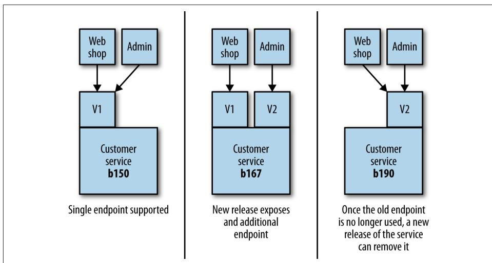
Figure 4-5. Coexisting different endpoint versions allows consumers to migrate gradually
